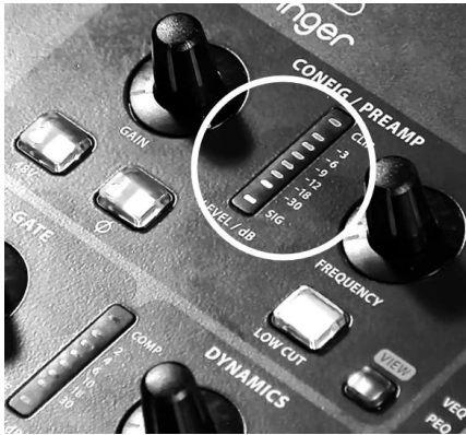
Too much gain, clipping the signal.
